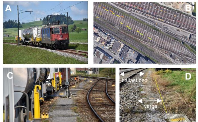
Fig 1: Photos of the hot water spray train (A, C), the surveyed area in Muttenz, CH (B) and an example for the treated track area (D).
