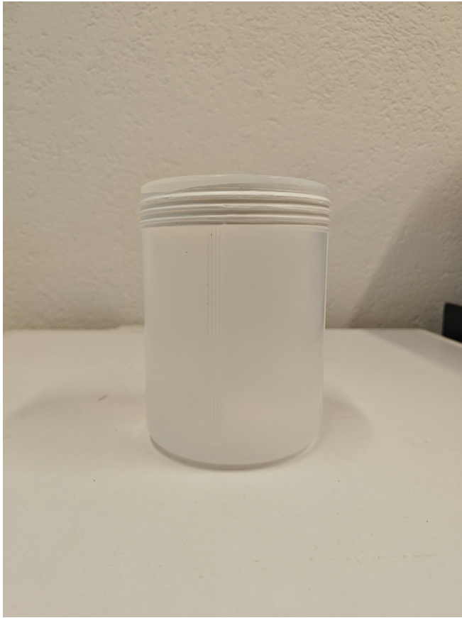
Fig. 2. Individual components of the dynamic flux multichamber system used to measure ammonia concentration in pig slurry replicates: (A) 1 L perfluoroalkoxy alkane jar, (B) perfluoroalkoxy alkane jar screw cap with two-quarter-inch tube ports, (C) cylinders and pressure regulator used to deliver synthetic air to the system, (D) 100 \mu\text{m} hole diameter critical orifices, (E) multichannel sampler, (F) cavity-ring down spectrometer and (G) jars in the water bath.
