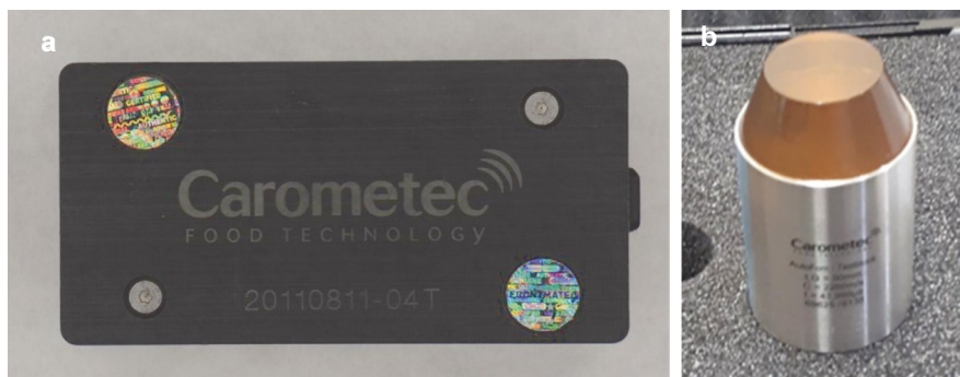
Fig. 11.2 Different types of patterns or "phantoms" for verifying carcass classification devices: (a) Pig plastic pattern for Fat-O-Meat'er (Frontmtec AS, DK), (b) Block for Autofom (Frontmtec AS, DK)
