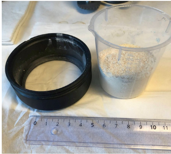
Fig. 7.1 Small sample cup from the FOSS DS2500 NIR scanner and a measuring cup containing the required amount of dried ground feed sample (~25 g) to adequately cover the bottom of the cup (Photo credit: Samantha Noel, Aarhus University, Denmark)
