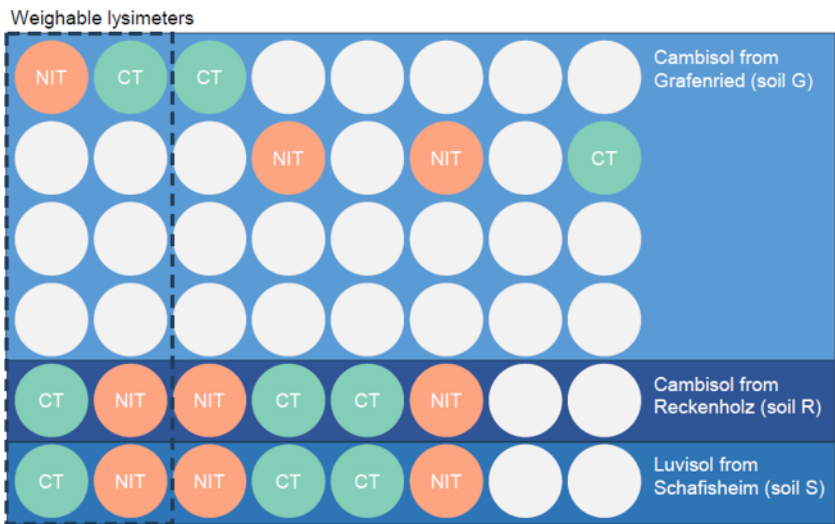
Figure A2. Experimental plan showing locations of treatments (CT = conventional tillage; NIT = non-inversion tillage) on lysimeter facility with soil monoliths from three locations in Switzerland.
