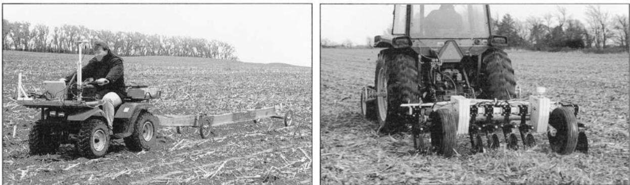
**Figure 1 Comparison of the electromagnetic and contact-based EC sensors in the field. (Left) Electromagnetic Geonics EM38 sensor (Right) Veris 3100 contact EC sensor. Source: (Sudduth et al., 2003).**
