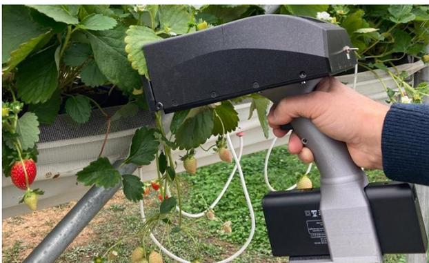
Figure 2: LeafEye device in use on site
