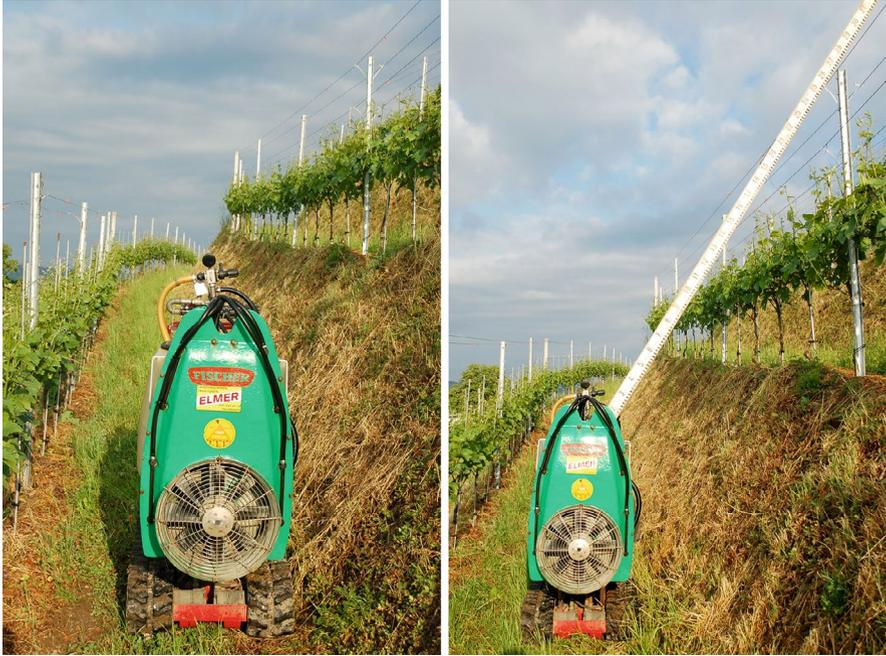
**Fig. 8.34** In steep vineyards, terraces allow the use of small tracked-vehicle-mounted axial fan sprayers (left). However, there are challenges in adapting the angle of the nozzles and air flow to reach the foliage hedge when the terrace slope is too steep (right)
