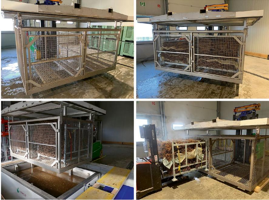
**Fig. 7.15** Hot-water treatment of grapevine plants in a specific device for maintaining the temperature precisely at 50 °C to destroy the phytoplasma and eggs of the flavescence dorée vector. (© Multiplants nursery, Vétroz, Switzerland)
