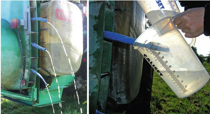
**Fig. 8.35** Flow rate is measured by placing rubber tubes over the nozzles to collect the spray in a graduated cylinder or container
