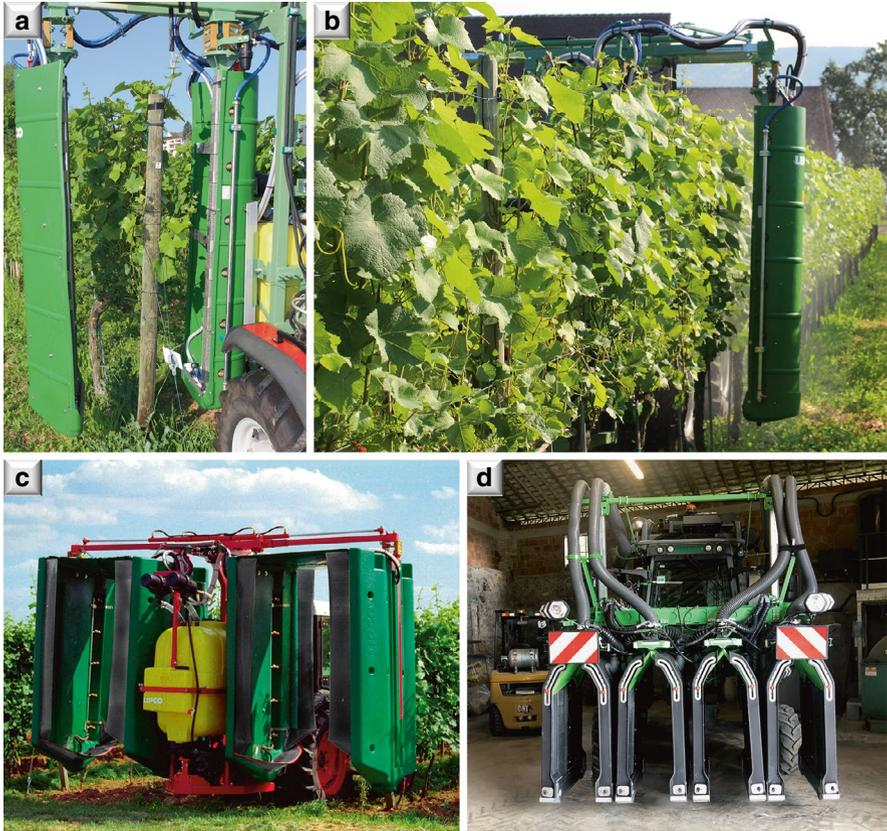
**Fig. 8.41** Tunnel sprayers with recycling techniques, which combine crossflow air assistance and nozzles (a, b), or those without air assistance (c), enable up to 30% of the spray volume to be recycled. Over-row tunnel sprayers are designed to simultaneously spray four rows of densely planted vineyards, as depicted in the Champagne region of France (d)
