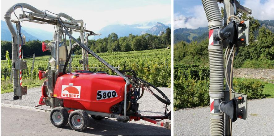
**Fig. 8.29** Pneumatic sprayers (left) can combine the presence of nozzles and a directed airflow to the canopy (right)
