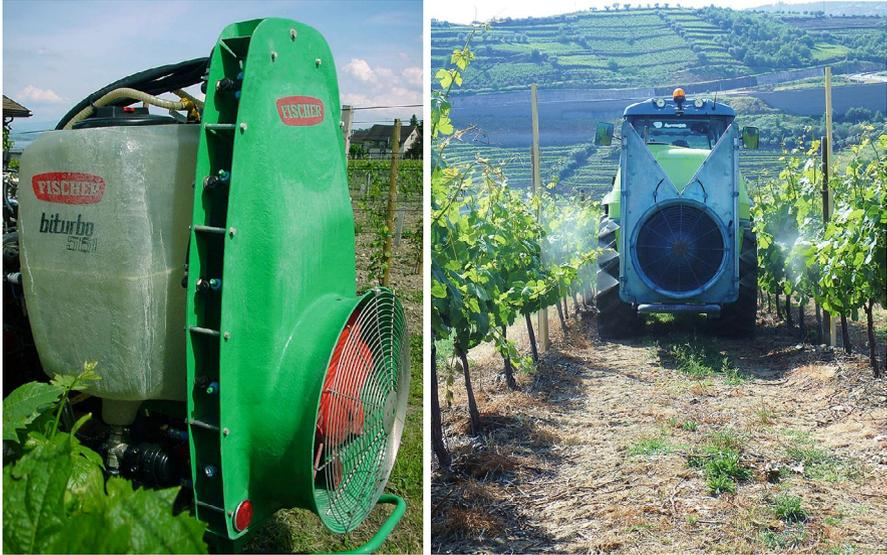
Fig. 8.24 Air-blast axial sprayers spread droplets generated by the nozzles to the foliage via airflow
