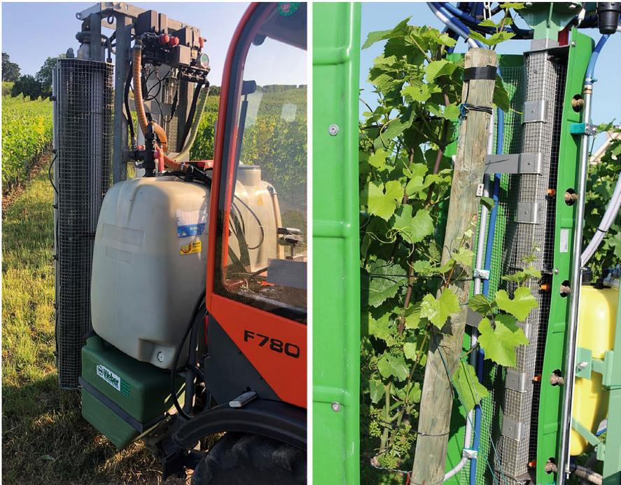
Fig. 8.25 Tangential or crossflow fans blow air horizontally onto the leaf canopy
