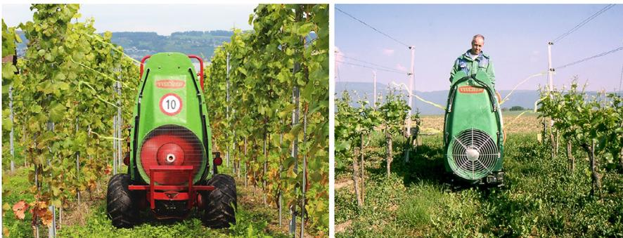
**Fig. 8.36** Properly oriented air- and spray flows are essential for optimising spray application. The angles of nozzles and deflectors should be precisely adjusted to the leaf canopy using thin tapes fixed on the nozzles
