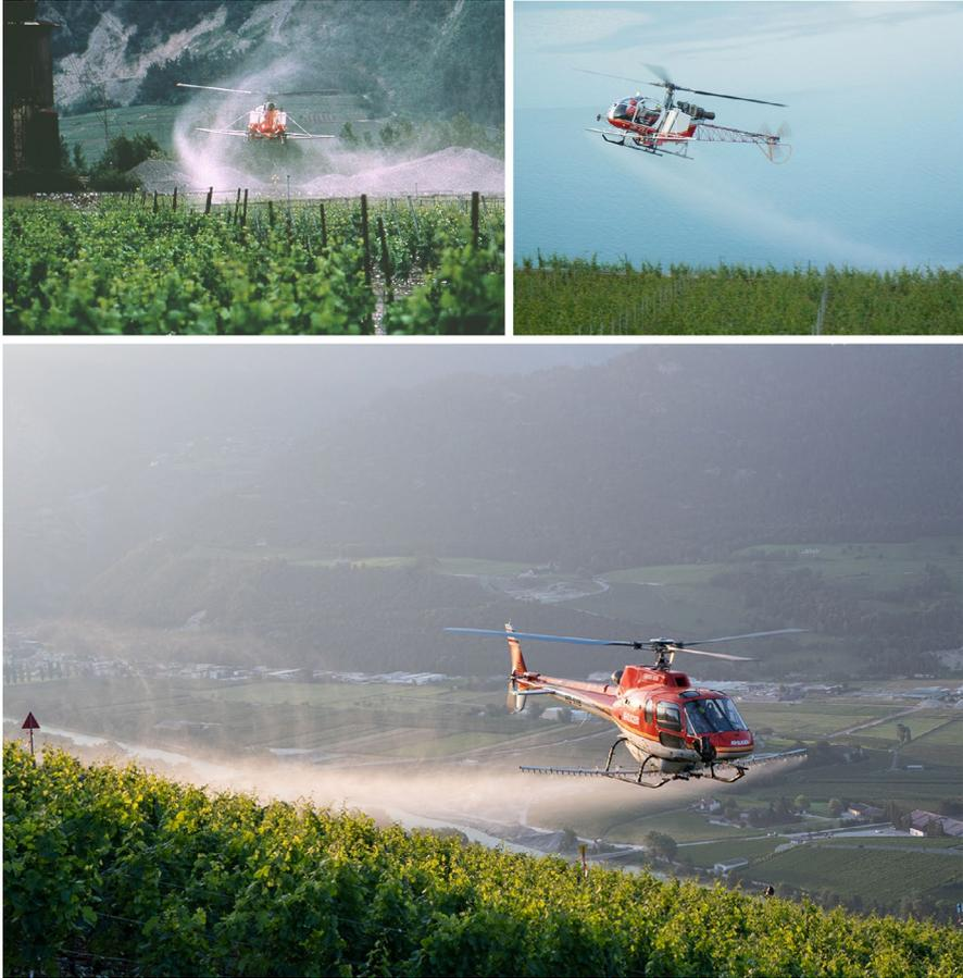
**Fig. 8.32** Although helicopters are very efficient at spraying vineyards they generate significant drift, and deposit and coverage inside the vine canopy is limited. Old Aerospatiale SA315B Lama (top left and right) generates noticeably higher drift than the modern Eurocopter Ecureuil AS350 B2 (bottom)
