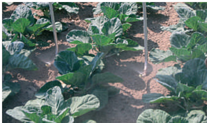
Droplegs fitted with Delavan hollow cone nozzles producing a spray angle of 115 degrees travel in the interrow space through a crop of Brussels sprouts.
