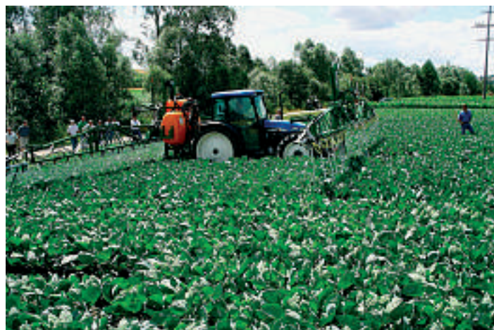
For contract spraying in Brussels sprouts and potatoes this tractor carries at the rear a 15m Amazone boom fitted with conventional flat fan or air injector flat fan nozzles, and in front a 15m Amazone boom fitted with 19 droplegs 120cm long with Delavan hollow cone nozzles.
