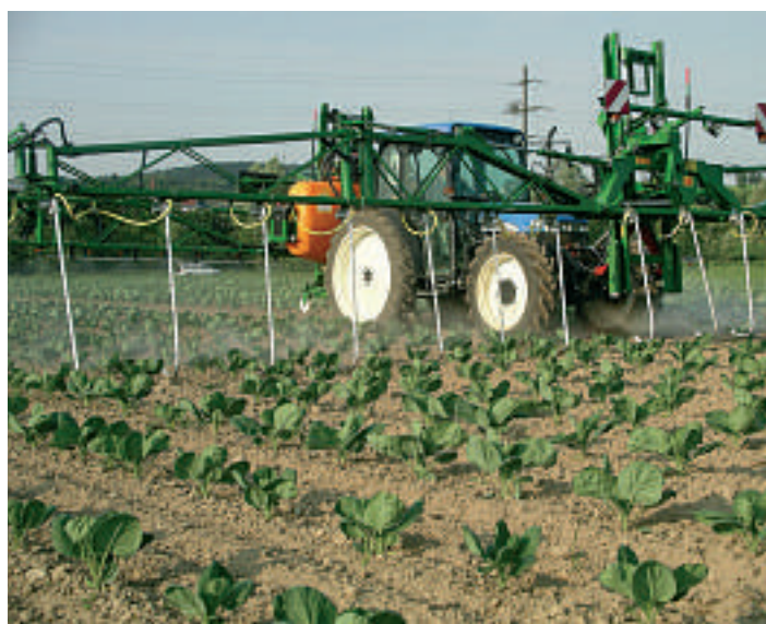
For contract spraying in Brussels sprouts and potatoes this tractor carries at the rear a 15m Amazone boom fitted with conventional flat fan or air injector flat fan nozzles, and in front a 15m Amazone boom fitted with 19 droplegs 120cm long with Delavan hollow cone nozzles.
