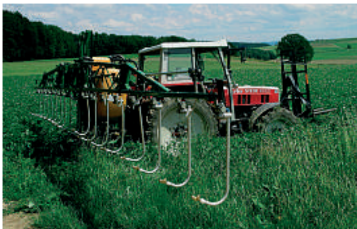
Droplegs with flat fan nozzles spraying sidewise or bottom up mounted on a 12m Amazone boom operated by an organic vegetable grower in potatoes, Brussels sprouts, cauliflower, and various cabbages in Switzerland. The same boom is also fitted with flat fan nozzles spraying top down.
