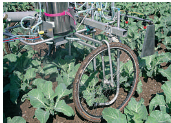
Field plot sprayer which carries in front on a horizontal bar conventional or air injector flat fan nozzles. Behind this bar droplegs are mounted which travel through the crop in the inter-row space. In onions each dropleg is fitted with two sidewise spraying flat fan deflector nozzles.
