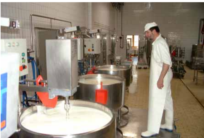
Production of model hard cheese (Gruyère type) in the pilot plant at Liebefeld.
