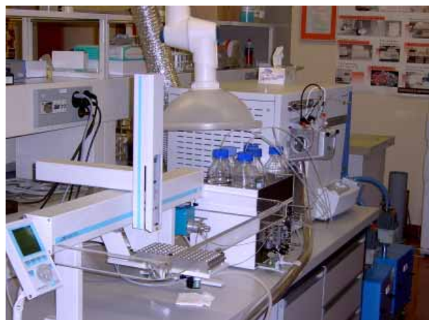
LC-MS apparatus for the quantification of bioactive peptides in Swiss cheese having an effect on blood pressure.
