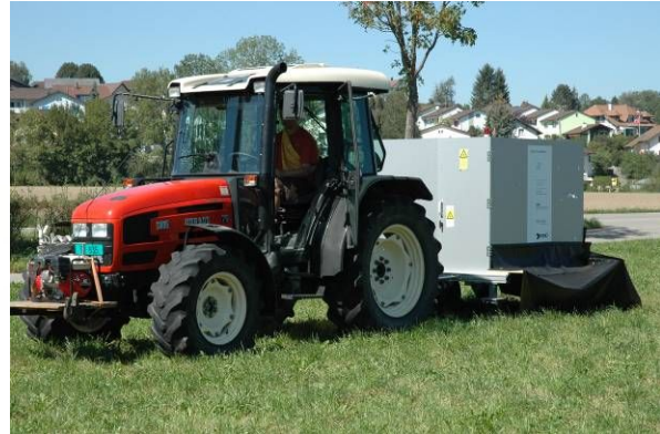
Fig. 2: Left: SmartWeeder processes 3D-images by means of a laser triangulation system. Right: SmartWeeder in action. The detected plants are sprayed by single nozzles. Source: Agroscope ART
