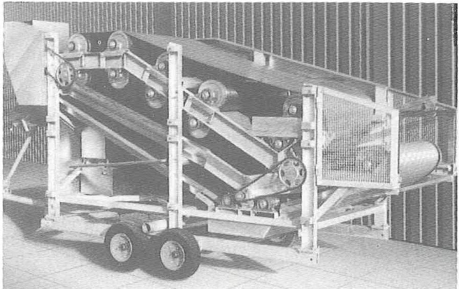
Abb. 3: Siebandpresse (mobile Anlage).
