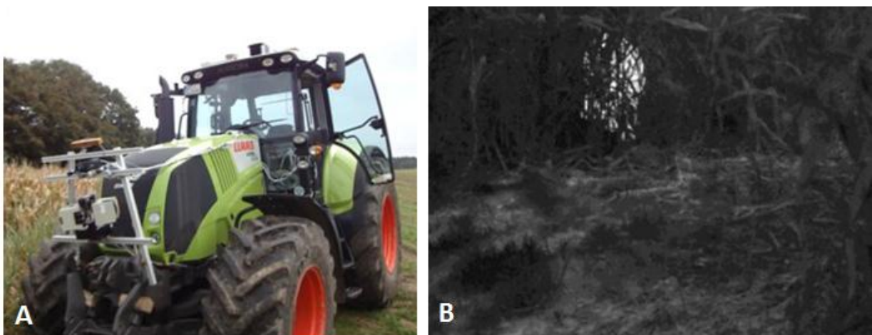
Ambient Awareness for Autonomous Agricultural Vehicles (QUAD-AV): Tractor with RADAR and odometer, rotating LIDARs, stereo cameras and thermographic camera (A); and view from a thermographic camera, in which a person hiding in a maize field is clearly visible (B). ICT-AGRI Project.
