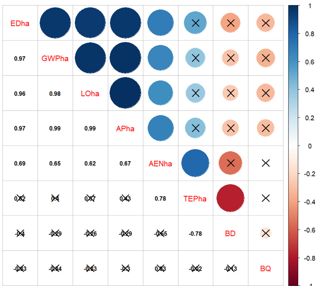
Fig. 3. Correlation matrix of environmental indicators. Results are based on the analysis of 12 pilot farms for 2016. EDha: energy demand per ha; GWPha: global warming potential per ha; LOha: land occupation per ha; APha: acidification potential per ha; AENha: aquatic eutrophication N per ha; TEPha: terrestrial ecotoxicity potential per ha; BD: biodiversity score; BQ: soil quality indicator. All environmental impacts except BD and BQ are per ha utilised agricultural area (UAA). Positive correlations are displayed in blue and negative correlations in red. Colour intensity and circle size are proportional to the correlation coefficients (see colour key on the right). Crosses indicate non-significant correlation coefficient at 95% confidence level. (For interpretation of the references to color in this figure legend, the reader is referred to the web version of this article.)
