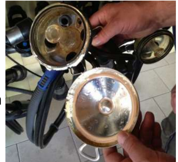
Deposits in the collection piece of the milking unit
