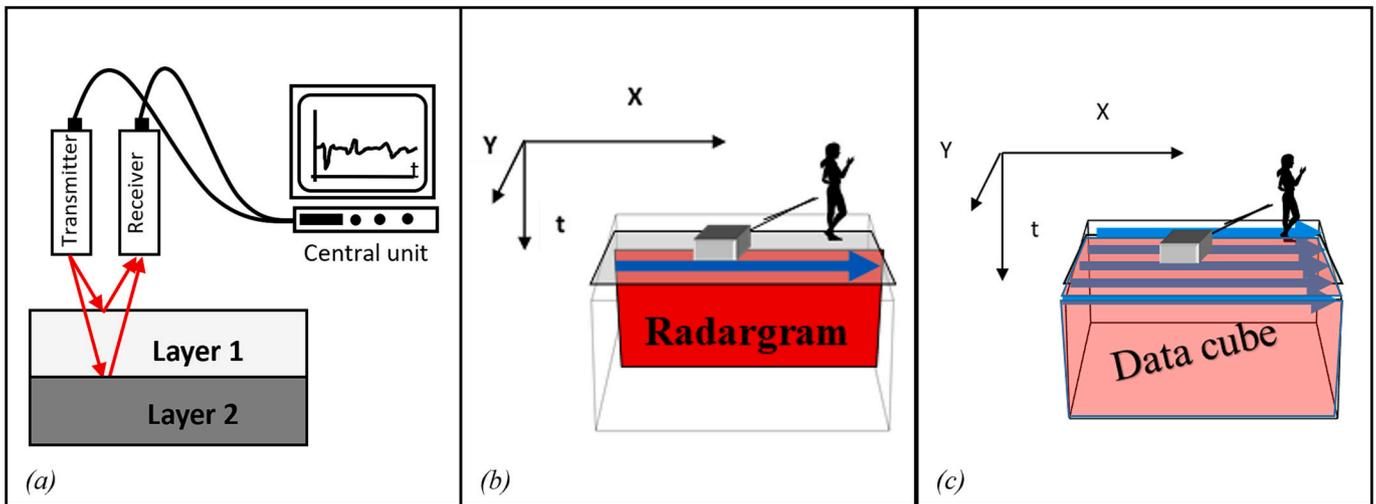
Fig. 2. (a) Principles of GPR with emitted and reflected signal (red arrows); (b) acquisition of a 2D dataset (radargram); (c) acquisition of a 3D datacube.
