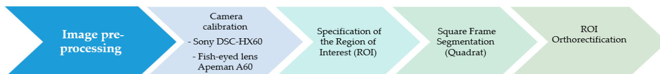
Figure 2. Structured Workflow for Image Preprocessing, covering all essential steps from defining the ROI to ensuring accurate orthorectification.
