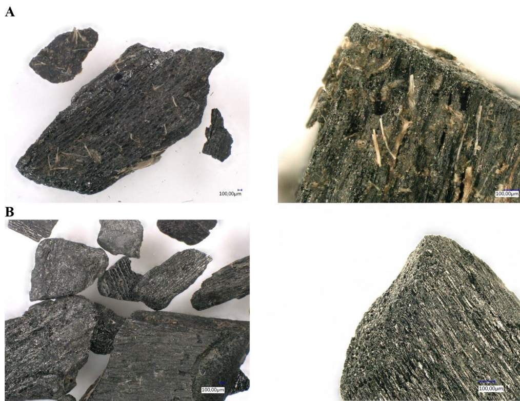
Fig. 1 Microscopy pictures of A digested biochar after washing with acetone and water, and B digested biochar after washing with acetone, water, and NaOH, Blue bars lower right corner indicate size scale of 100 \mu\text{m}
